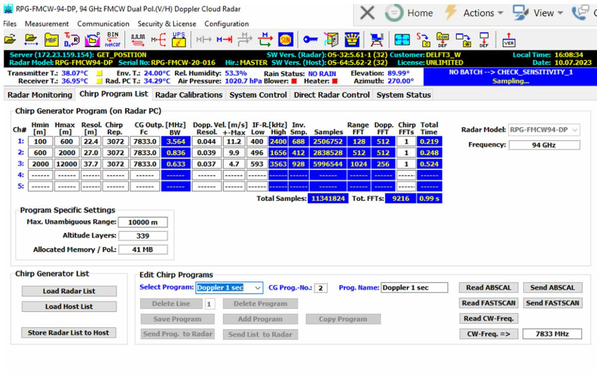
**Figure 2: Illustrative Chirp Tables for a Dual-Frequency RPG Radar.** This figure presents examples of chirp tables designed for a dual-frequency RPG radar, featuring configurations for both 35 GHz (top) and 94 GHz (bottom) frequencies. While most specifications remain consistent across both frequencies, notable adjustments are primarily observed in the Doppler velocity parameters, including maximum values and resolution.
