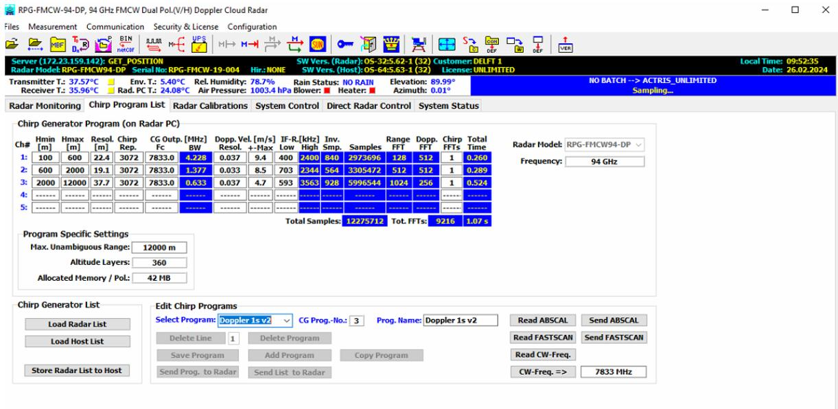
**Figure 1: Illustrative Chirp Table for an RPG Radar Operating at 94 GHz.** This figure depicts an example chirp table tailored for an RPG radar operating at 94 GHz, specifically designed for Plan Position Indicator (PPI) mode to derive vertical profiles of horizontal wind. The elevation angle for PPI mode is set at 85°. Parameters displayed in the white columns are adjustable manually to accommodate specific measurement requirements.
