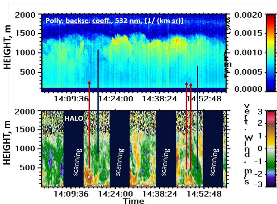
Figure 13: Synchronized dataset of PollyXT data (top) and HALO Doppler lidar (bottom).
