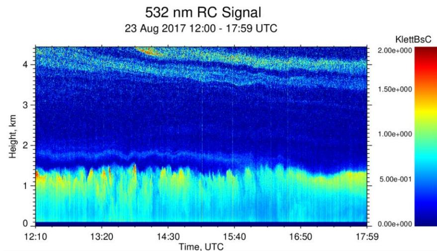
Figure 1: Particle backscatter coefficient at 532 nm derived from the newly installed analogue detector with the Klett-method for Polly XT operating at Košetice on 23 Aug 2017. The temporal and spatial resolution is 5 s and 7.5 m respectively.
