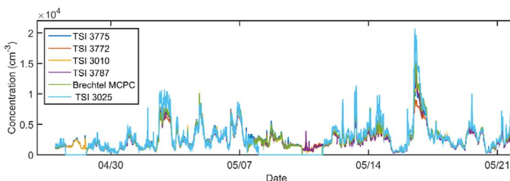
Figure 1. Time series of particle number concentration measured with the different CPCs over the measurement campaign 24 April – 22 May 2017 at the Hyytiälä Forestry field station.
