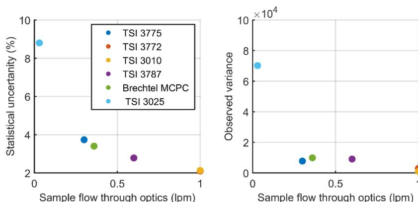
Figure 2. Mean statistical uncertainty of the recorded concentration and observed variance as a function of sampled aerosol flow.
